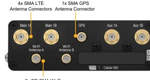
2x RP-SMA Wi-Fi Antenna Connectors
