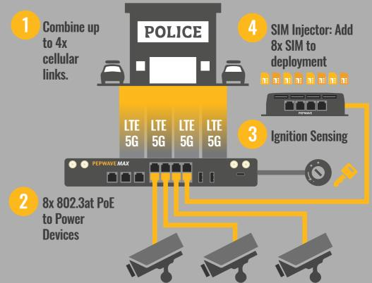
The HD4 MBX combines the bandwidth of 4x Gigabit LTE links into a fast, reliable, and secure SD-WAN connection, enabling you to stream high-definition video in real-time. This can all be achieved without investing in any infrastructure. With SpeedFusion-enabled devices on multiple vehicles and aerial resources, you can monitor the situation from multiple perspectives without needing a line-of-sight connection.
